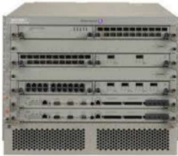
Core aggregation switch in Central Office/POI Aggregates traffic to pass to Retailers
