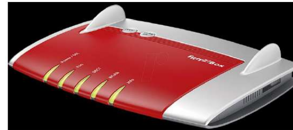
Retailer router connects to ONU with Ethernet cable provides voice, Wi-Fi & internet in the home
